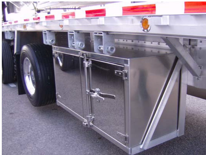
Example of support brackets
